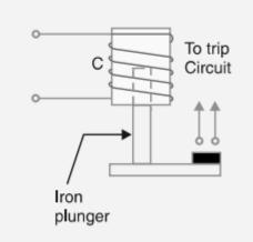
When a fault occurs the current through the relay coil becomes more than the pickup value, causing the plunger to be attracted to the solenoid. The upward movement of the plunger closes the trip circuit, thus opening the circuit breaker and disconnecting the faulty circuit.
