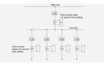
➢ If the faults are not cleared by primary relay system because of trouble within the relay, wiring system or breaker. Under such conditions, back-up protection does the required job.
