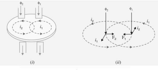
and  $i_{2} \propto \phi_{1max} \cos \omega t$  $i_{2} \propto \frac{d\phi_{2}}{dt} \propto \phi_{2max} \cos (\omega t + \alpha)$ Now,  $F_{1} \propto \phi_{1} i_{2} \text{ and } F_{2} \propto \phi_{2} i_{1}$
