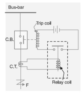
The relay circuit connections can be divided into three parts
