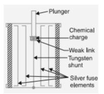
➤ When a fault occurs, the silver fuse elements are the first to be blown out and then current is transferred to the tungsten wire. The weak link in series with the tungsten wire gets fused and causes the chemical charge to be detonated. This forces the plunger outward to operate the circuit breaker. The travel of the plunger is so set that it is not ejected from the fuse body under fault conditions.
