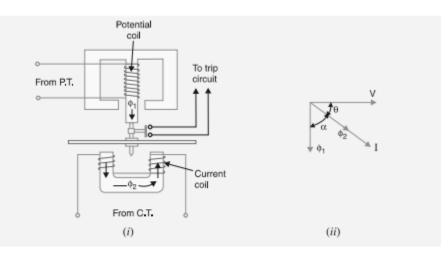
The interaction of fluxes  $\phi_1$  and  $\phi_2$  with the eddy currents induced in the disc produces a driving torque given by :
